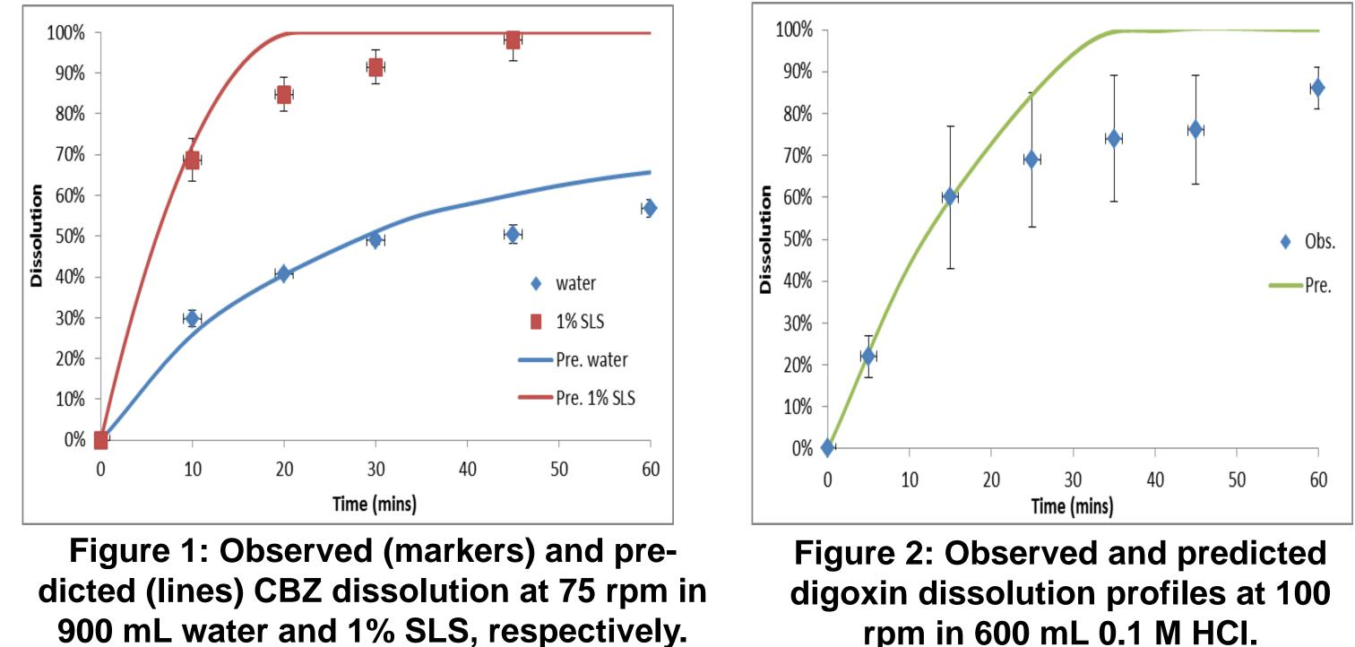
The aim herein is to model drug particle dissolution in the USP 2 paddle apparatus using a combination of particle motion and the Noyes-Whitney equations<sup>3</sup>.
