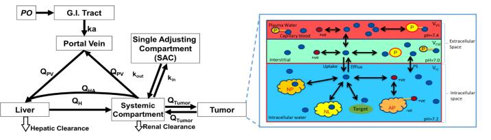
Left panel: Q<sub>H</sub>, Q<sub>PV</sub>, Q<sub>HA</sub>, and Q<sub>Tumor</sub> are blood flows in the liver, portal vein, hepatic artery, and tumor, respectively; k<sub>in</sub> and k<sub>out</sub> are first-order rate constants that act on the masses of drug within the systemic compartment and the single adjusting compartment, respectively.
